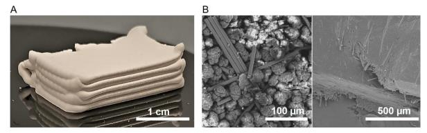
**Principle of direct gel printing:** aqueous formulations of thermoplastic powders, fillers and binder form a matrix with specific rheological properties (yield stress fluid) that can be printed in multilayers. (A) Deposit after drying of 5 layers of a dispersion of polymer (confidential) powder (10 µm grains, approximately 2 mm thick layers). (B) Example of formulation of PA12 powder and carbon fibers before and after thermal annealing.
